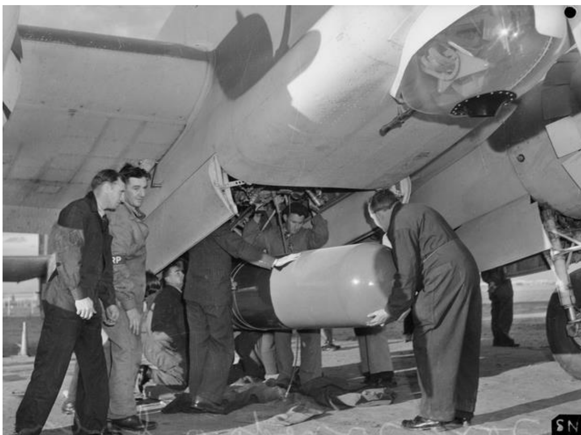
Figure 15. Employees of the Commonwealth Aircraft Corporation fitting a practice torpedo into the bomb bay of a Beaufort Bomber, Melbourne June 1942. (Australian War Memorial)
